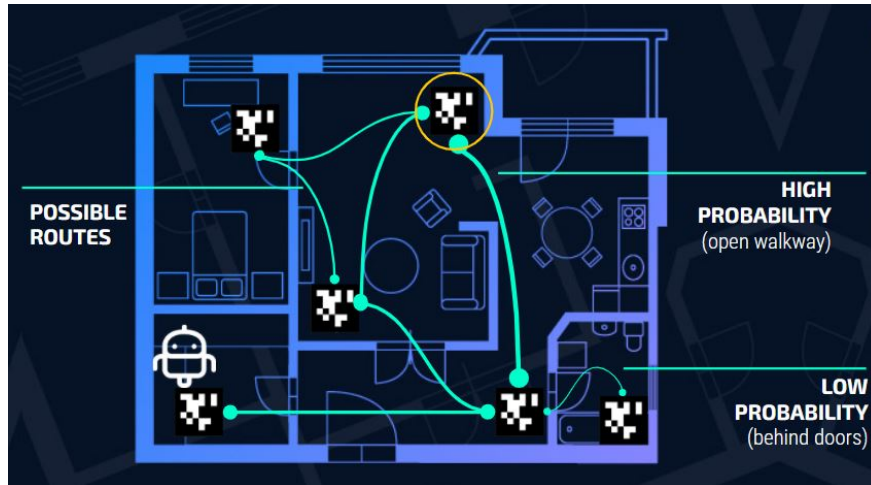
Figure 2: Each possible route for the robot is labeled with an edge, whose thickness represents the probability that edge is traversable at any given time
